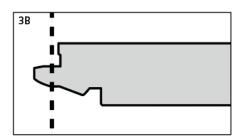
Begin the first row with a whole plank. First saw off the tongue on both the long and the short sides. **See diagram 3B.**
