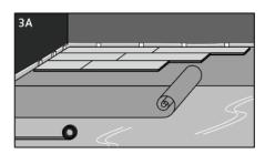
First install the underlayment, per width and gradually as you progress. If the underlayment is pre-mouted on the panels, then you can skip this step. **See diagram 3A**.
