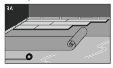
First install the underlayment, per width and gradually as you progress. If the underlayment is pre-mouted on the panels, then you can skip this step. **See diagram 3A.**
