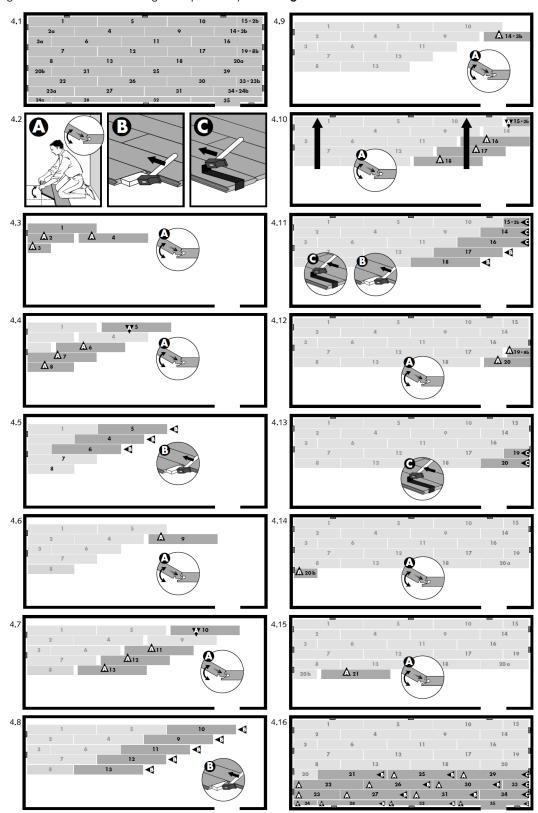
In places where it is too difficult to install the Uniclic planks with the tapping block (e.g. against the wall), you can tap them together using the crowbar and a hammer. **See diagrams 5A - 5B - 5C.**
