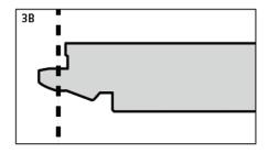
Begin the first row with a whole plank. First saw off the tongue on both the long and the short sides. **See diagram 3B.**
